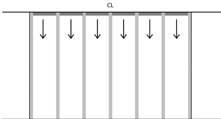
6. Place horizontal furring strips 23 1/2" apart starting at the top of the wall working downward.
