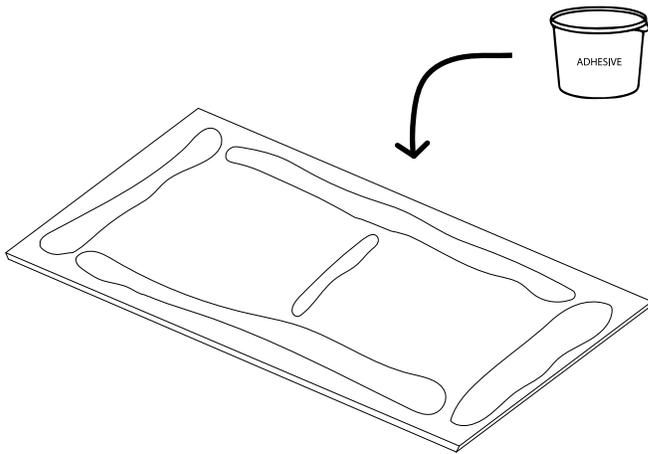
9. Take the first BRIK and align it properly on the furring strip. Use construction adhesive at the location of the furring strip.
